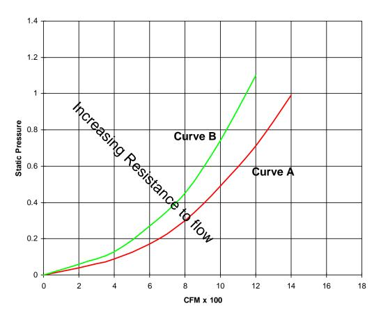
Going from curve A to curve B is an example of a system that a damper closes or filters get dirty.
