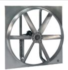
Designed for commercial and industrial applications requiring both exhaust and supply air. Construction includes rigid drive frame rails and one-piece motor/bearing plate. Propeller utilizes a six-blade cast aluminum design which provides low sound levels. Fans may be mounted either in the horizontal or vertical positions.
