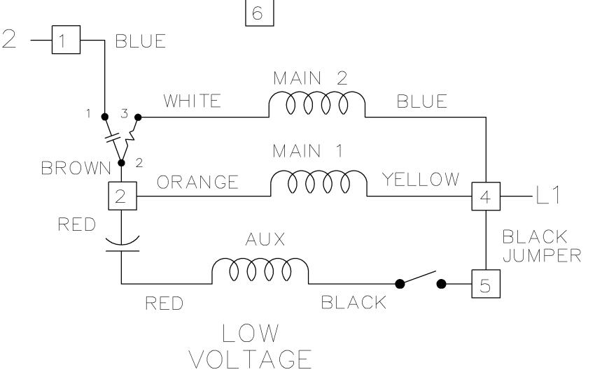
DUAL VOLTAGE CAPACITOR START REVERSIBLE ON TERM BOARD WITH OVERLOAD PROTECTION
