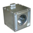
Designed for indoor clean air applications including intake, exhaust, return, or make-up air systems in industrial or commercial buildings. Rugged construction allows fan to be installed in ductwork either horizontally or vertically. Duct collars provide easy duct connections
