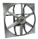
Designed for commercial and industrial applications requiring high volume of air at low to medium static pressures. Construction includes heavy-duty drive frame channels, bearing plate and motor plate. Propeller utilizes a six-blade heavy-duty cast aluminum design. Mount in vertical position for exhaust applications or horizontal position for supply applications.
