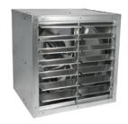
Designed for commercial and industrial applications requiring assembled packaged units able to deliver high volumes of air at low static pressures. Fans are completely assembled and ready for installation. Construction includes galvanized steel fan panel, fabricated propeller and bolted cabinets. Fan includes wall mounting angles for easy installation.
