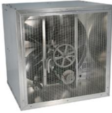
Designed for commercial and industrial applications requiring assembled packaged units able to deliver high volumes of air at low static pressures. Fans are completely assembled and ready for installation. Construction includes galvanized steel fan panel, fabricated propeller and bolted cabinets. Fan includes wall mounting angles for easy installation.
