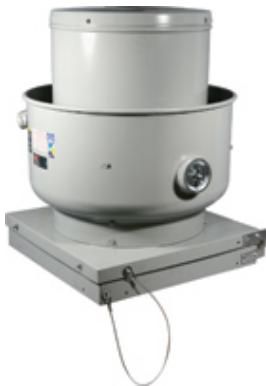
Designed for heavy grease applications as found in char broilers, solid fuel cooking, and Oriental cooking. Fans are UL 762 listed for all electrical components and grease removal. Units are constructed of heavy gauge steel and utilize a one-piece steel windband that is continuously welded to the curb cap. Clean out port, heat baffle, Nema-1 junction box, and hinged base are included.
