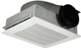
Low profile, high performance exhaust ventilators designed for residential, commercial, institutional and industrial applications. Factory assembled for side discharge for installation in ceilings. Constructed of galvanized steel and a molded white polystyrene, easy-to-clean grille. Hardware and mounting brackets are included.
