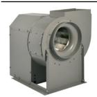
Designed for commercial kitchen exhaust or industrial spark resistant applications requiring high volumes of air at high static pressures. Suitable for ducted exhaust, supply or return-air applications. Constructed out of heavy gauge steel with polyester gray coating. The scroll is welded, has a bolted access door and 1 inch threaded drain connection for easy cleaning.
