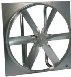
Designed for commercial and industrial applications requiring high volumes of air at low static pressures. Construction includes rigid drive frame rails and one-piece motor/bearing plate. Mount fan in vertical position for exhaust applications or horizontal position for supply applications.
