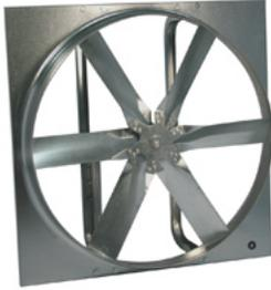
Designed for commercial and industrial applications requiring high volumes of air at low static pressures. Construction includes rigid drive frame rails and one-piece motor/bearing plate. Mount fan in vertical position for exhaust applications or horizontal position for supply applications.
