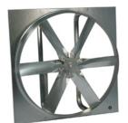
Designed for commercial and industrial applications requiring high volumes of air at low static pressures. Construction includes rigid drive frame rails and one-piece motor/bearing plate. Mount fan in vertical position for exhaust applications or horizontal position for supply applications.
