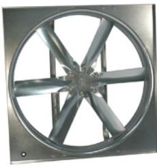
Designed for commercial and industrial applications requiring high volumes of air at low static pressures. Construction includes rigid drive frame rails and one-piece motor/bearing plate. Mount fan in vertical position for supply applications or horizontal position for exhaust applications.
