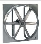
Designed for commercial and industrial applications requiring both exhaust and supply air. Construction includes rigid drive frame rails and one-piece motor/bearing plate. Propeller utilizes a six-blade cast aluminum design which provides low sound levels.
