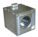
Designed for indoor clean air applications including intake, exhaust, return, or make-up air systems in industrial or commercial buildings. Rugged construction allows fan to be installed in ductwork either horizontally or vertically. Duct collars provide easy duct connections. Energy Saving units feature EC motors which allow up to 80% usable turndown. Motor features potentiometer dial for speed adjustment. Optional Variable-Speed Control Kit (43Y140) can be used to remotely control speed.
