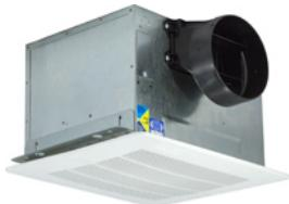
Insulated, quiet, high performance exhaust ventilators designed for residential, commercial, institutional and industrial applications. Factory assembled for horizontal discharge. Constructed of galvanized steel and a molded white polystyrene, easy-to-clean grille. Hardware and mounting brackets are included.
