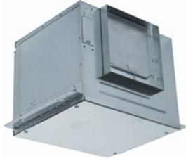
High performance exhaust ventilators designed for residential, commercial, institutional and industrial applications. Factory assembled for horizontal discharge but can be rotated to vertical discharge in the field. Constructed of galvanized steel with a removable access panel on the bottom of unit. Hardware and mounting brackets are included.
