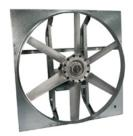
Designed for commercial and industrial applications requiring high volume of air at low to medium static pressures. Construction includes heavy-duty drive frame channels, bearing plate and motor plate. Propeller utilizes a six-blade heavy-duty cast aluminum design. Mount in vertical position for exhaust applications or horizontal position for supply
