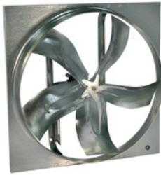
Designed for commercial and industrial applications requiring high volumes of air at low static pressures. Construction includes heavy-duty drive frame rails and one-piece motor/bearing plate. Propeller utilizes a five-blade reinforced galvanized steel design which provides low sound levels. Mount in vertical position for exhaust applications or horizontal position for supply applications.
