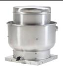
Designed for use in schools, commercial, and industrial applications to exhaust clean air, up and away from the roof. Leakproof, spun aluminum construction features a fully rolled windband for increased stability. Energy Saving units feature EC motors which allow up to 80% usable turndown. Motor features potentiometer dial for speed adjustment.
