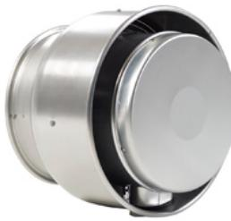
Designed for use in schools, commercial, and industrial applications to exhaust clean air, up and away from the building. Leakproof, spun aluminum construction features a fully rolled windband for increased stability. Energy Saving units feature EC motors which allow up to 80% usable turndown. Motor features potentiometer dial for speed adjustment. Optional Variable-Speed Control Kit (43Y140) can be used to remotely control speed.
