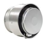
Designed for use in schools, commercial, and industrial applications to exhaust clean air, up and away from the building. Leakproof, spun aluminum construction features a fully rolled windband for increased stability. Energy Saving units feature EC motors which allow up to 80% usable turndown. Motor features potentiometer dial for speed adjustment. Optional Variable-Speed Control Kit (43Y140) can be used to remotely control speed.
