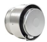
Designed for use in restaurants, schools, commercial, and industrial applications to exhaust contaminated air from kitchen range hoods, up and away from the building. Leakproof, spun aluminum construction features a fully rolled windband for increased stability. Energy Saving units feature EC motors which allow up to 80% usable turndown. Motor features potentiometer dial for speed adjustment. Optional Variable-Speed Control Kit (43Y140) can be used to remotely control speed.
