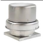
Designed to meet the general clean air exhaust requirements for industrial and commercial buildings. Features a fully rolled windband bead for increased stability and easy transport. Fresh outside air is drawn in under the motor cover to maximize motor life. Energy Saving units feature EC motors which allow up to 80% useable turndown. Motor features potentiometer dial for speed adjustment. Optional Variable-Speed Control Kit (43Y140) can be used to remotely control speed.
