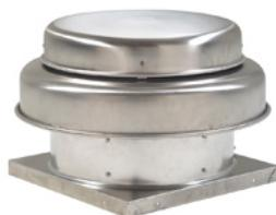
Designed for situations requiring the steady exhaust of air under low to moderate static pressures. Fully rolled baffle bead for stability and ease of transport with spun aluminum hood construction. Galvanized steel venturi, inlet and supports.
