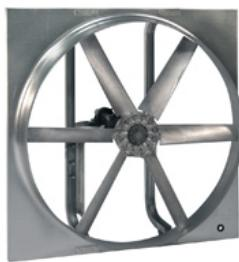
Designed for commercial and industrial applications requiring both exhaust and supply air. Construction includes rigid drive frame rails and one-piece motor/bearing plate. Propeller utilizes a six-blade cast aluminum design which provides low sound levels. Fans may be mounted either in the horizontal or vertical positions.
