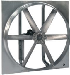
Designed for commercial and industrial applications requiring both exhaust and supply air. Construction includes rigid drive frame rails and one-piece motor/bearing plate. Propeller utilizes a six-blade cast aluminum design which provides low sound levels. Fans may be mounted either in the horizontal or vertical positions.
