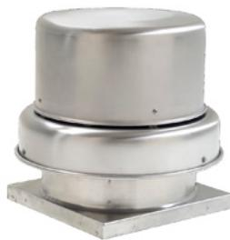
Designed for situations that require steady exhaust of clean air under low-to-moderate static pressures. Spun aluminum construction including a fully rolled bead on the windband, ensures stability and provides rigidity for lifting and transporting.
