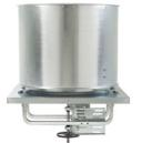
Designed for use in industrial and commercial buildings such as warehouses, manufacturing facilities, foundries, and laboratories. Housing is constructed of heavy gauge galvanized steel. The windband is removable for easy inspection. Lifting lugs are provided.
