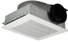
Low profile, high performance exhaust ventilators designed for residential, commercial, institutional and industrial applications. Factory assembled for side discharge for installation in ceilings. Constructed of galvanized steel and a molded white polystyrene, easy-to-clean grille. Hardware and mounting brackets are included.
