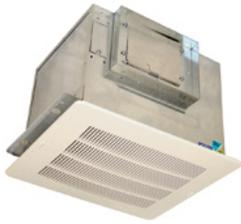
Insulated, quiet, high performance exhaust ventilators designed for residential, commercial, institutional and industrial applications. Factory assembled for horizontal discharge but can be rotated to vertical discharge in the field. Constructed of galvanized steel and a molded white polystyrene, easy-to-clean grille. Hardware and mounting brackets are included.
