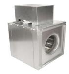
Designed for indoor clean air applications including intake, exhaust, return, or make-up air systems in industrial or commercial buildings. Rugged construction allows fan to be installed in ductwork either horizontally or vertically. Duct collars provide easy duct connections. Access panels are included on each side of the unit.
