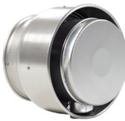
Designed for use in restaurants, schools, commercial, and industrial applications to exhaust contaminated air from kitchen range hoods, up and away from the building. Leakproof, spun aluminum construction features a fully rolled windband for increased stability. Energy Saving units feature EC motors which allow up to 80% usable turndown. Motor features potentiometer dial for speed adjustment. Optional Variable-Speed Control Kit (43Y140) can be used to remotely control speed.
