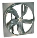
Designed for commercial and industrial applications requiring high volumes of air at low static pressures. Construction includes heavy-duty drive frame rails and one-piece motor/bearing plate. Propeller utilizes a five-blade reinforced galvanized steel design which provides low sound levels. Mount in vertical position for exhaust applications or horizontal position for supply applications.
