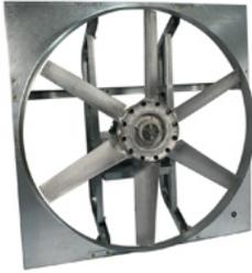
Designed for commercial and industrial applications requiring high volume of air at low to medium static pressures. Construction includes heavy-duty drive frame channels, bearing plate and motor plate. Propeller utilizes a six-blade heavy-duty cast aluminum design. Mount in vertical position for exhaust applications or horizontal position for supply applications.
